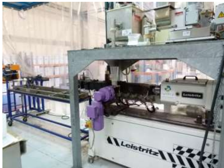
Figure 1. Leistritz extruder from Gaiker.
