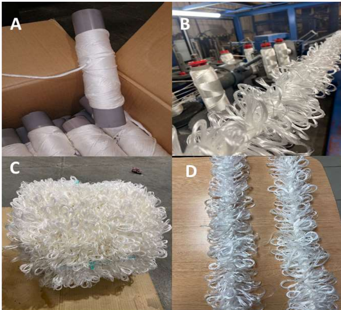
Figure 7 Sequence of the rope prototype production, using multifilament bobbins (A) at industrial rope manufacturing machine at Itsaskorda's (B), to obtain rope with characteristics of commercial counterparts (C) and finally cut down to the length for mussel suspended culture (D).
